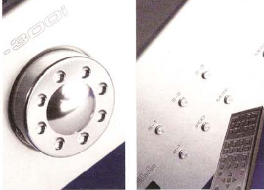
ABOVE: No simple volume control but a rotary encoder that navigates through the input, balance and volume menu options
