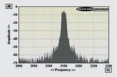
ABOVE: Wow and flutter re. 3150Hz tone at 5cm/sec (plotted  $\pm 150$ Hz, 5Hz per minor division). Note very low rate drift as the W&F signal is averaged over time
