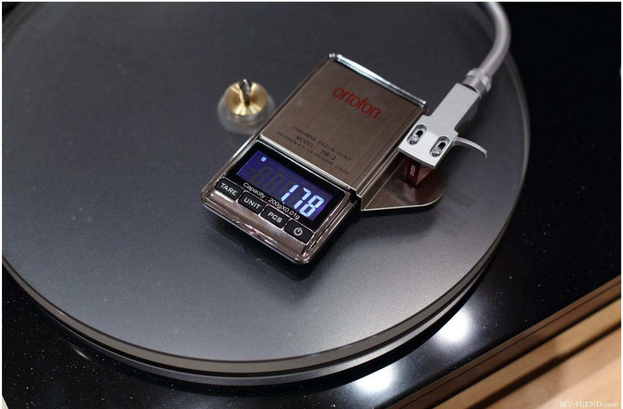
Re-adjust the MC cartridge after replacing it.
