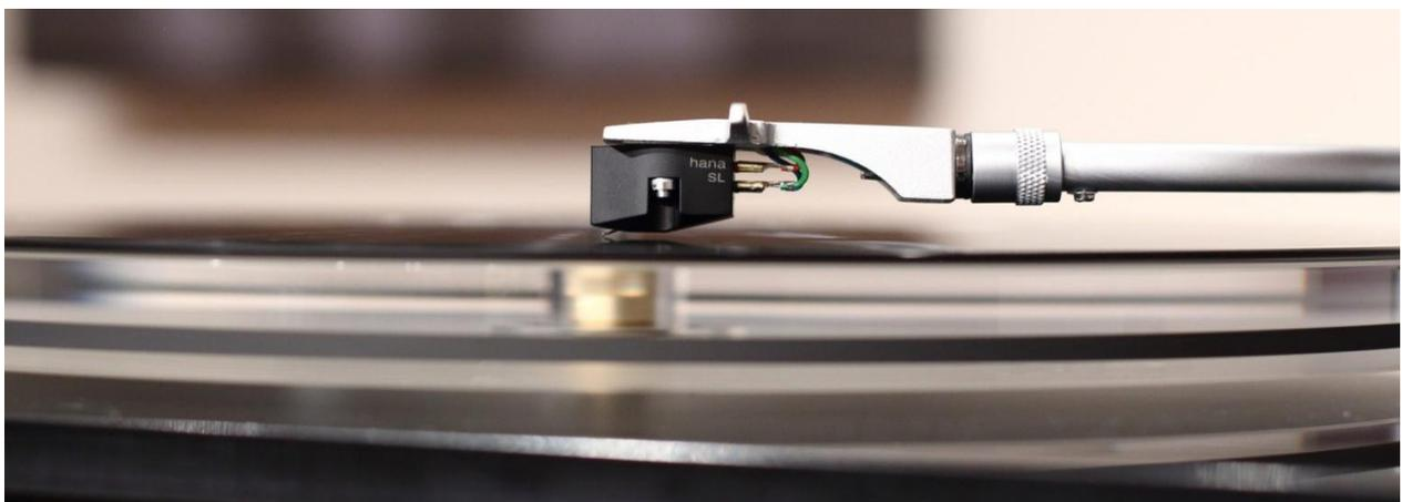
Degaussing is only applicable to MC cartridges. If you are using the original standard MM cartridge, it is not required.
