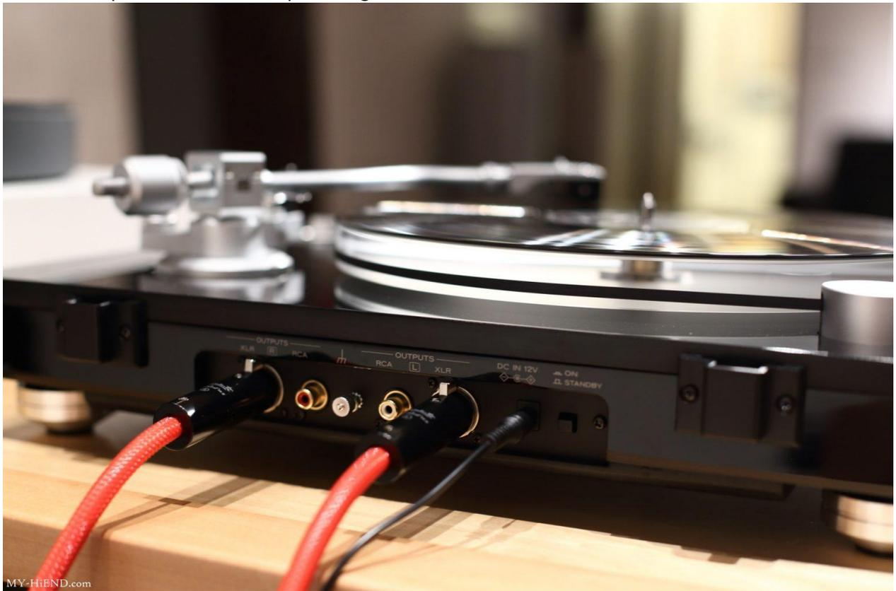
The space between the input and output of the PE-505 is quite large, so it is no problem to use fewer wires with larger terminal diameters.
