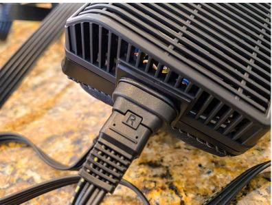
the good. The cable, which was formerly permanently attached, is now unplug-able and easily replaced. Headphone cables get strain during their daily use, and this is a most welcome change.
