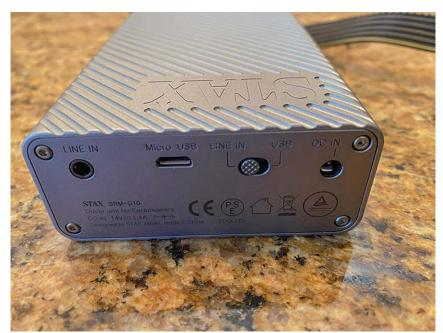
Getting started with the headphones is simple enough. First, charge the SRM-D10 Amplifier. A small LED glows red when the unit is charging, and turns off when charging is complete. Unattached to its charging cable, the LED glows green while it is in use. There is a power/volume control which feels high in quality.
