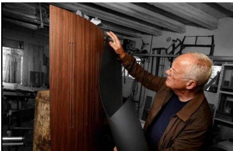
Serblin, by all accounts, was meticulous about the design and build of his speakers. The Accordos are made from solid walnut with the wood dried up to six months to attain correct stability. Even the brilliant chrome treatments are adhered chemically in the Vicenza factory. Back to set up. Serblin is specific about the 'chord' (in Accordo) and explains it:
