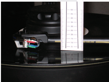
Measuring VTA with the SME protractor.
