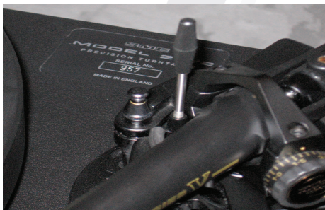
The tall guy with the rubber end-cap is the VTA screw.
