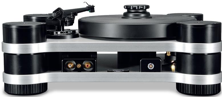
**ABOVE:** The 90° swivel joint at the base of the Series V tonearm is replaced in the Series VA with captive leads that feed a pair of gold-plated RCA outputs. A separate LEMO socket connects to the outboard speed controller via a screened umbilical
