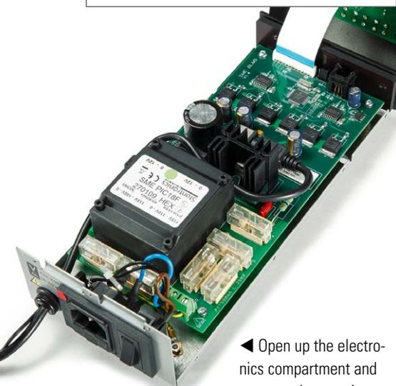
◀ Open up the electronics compartment and you reveal expensive components used for the supply and control of the drive motor.
