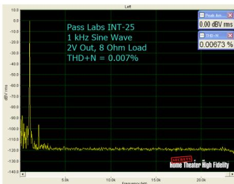
The first test I ran on the INT-25 was a 1 kHz sine wave at 2V RMS into a static 8 Ω load. THD+N measured just 0.007%. I can see the 2 kHz harmonic and can just barely make out the 3 kHz harmonic until all other harmonics disappear into the very low noise floor. This low contribution of higher-order harmonic distortion is a major design goal of Mr. Colburn and is demonstrated in the tests I performed.
