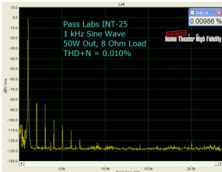
Increasing the output to twice the rated power, or 50 Watts into 8  $\Omega$ , the THD+N remained well below the threshold of audibility at just 0.010%. Compare this reading to the manufacturers claim of 0.1% for the 25 Watt rated power into an 8  $\Omega$  load. The actual production amplifier I reviewed produces at least twice the power than the manufacturer's claim. I did not push it any further on this test.
