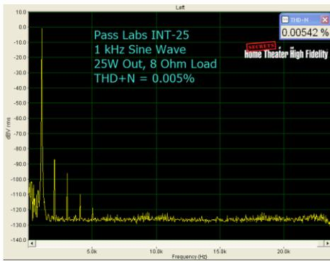
The INT-25 tested at its rated power of 25 Watts into 8  $\Omega$  presents a very clean and orderly distortion profile. The calculated THD+N is just 0.005%.
