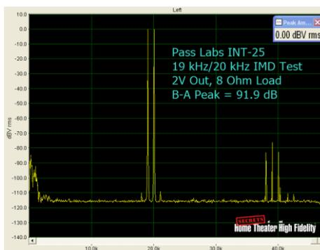
This is the other IMD Test we run with signals at 19 kHz and 20 kHz at equal gain. The B-A peak is the difference between the test signal and the level of the 1 kHz tone generated in sympathy to the two test tones. I measured this on-screen and got a B-A peak response of -91.9 dB at 2 Volts output.
