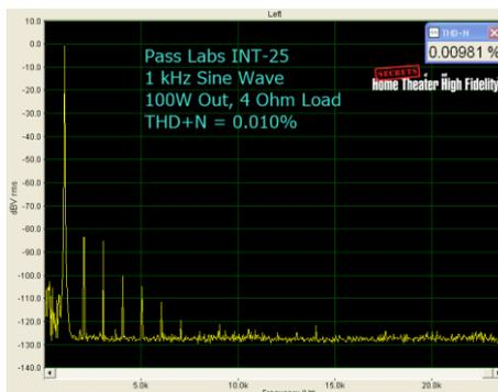
The INT-25 is similarly rated to put out a clean 50 wpc into a 4  $\Omega$  load. Well, with the above test, I doubled that number and again the distortion was only 0.010%. Excellent!
