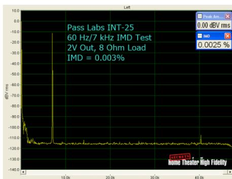
This next test is the Intermodulation Distortion Test with signals at 60 Hz and 7 kHz at a 4:1 ratio. The INT-25's measured IMD at 6 dBV (2 Volts) came to just 0.003%.
