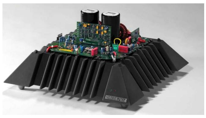
these amplifiers, I could barely get them to become warm to the touch. The amplifier also sports blue LEDs that flash in brightness proportionate to the amount of power the amplifier is generating. Red, which I only managed to trigger once, signals that the amplifier is clipping. If the amplifier is unduly stressed, it will terminate operation before the loudspeaker is damaged.
