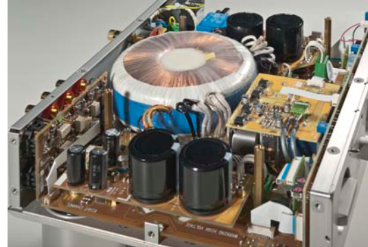
Nagra 300i: internal view of the right side
