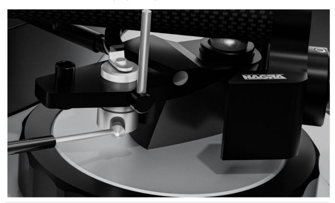
The tonearm's bearing is a simple, extremely precise, CNC machined, hardened steel cone captured in a resonance isolating, silicone damped, ultra high density polyethylene receiving cup. The tonearm's traditional counterweight is supplemented by a low hung, saddle shaped weight providing stability while minimising the tonearm's effective mass.
