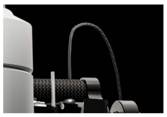
Vertical tracking angle of the cartridge is an extremely important alignment parameter. Users of the Reference Anniversary turntable/tonearm will enjoy the ability to easily and repeatably adjust VTA "on the fly". An oversized, high precision, rotary collar facilitates smooth, exactingly fine adjustments, as with a Leica camera lens. This system permits up to 10 mm/.4 in. of vertical travel.
