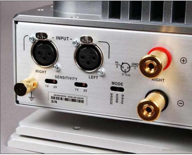
A bridge selector switch on the rear allows parallel bridging to double output current as well as power. A small toggle switches between bridge, normal and bi-amp modes. There are also two small switches to change input sensitivity between 1 and 2V. Finally there's the IEC power inlet and a mechanical on/off switch.
