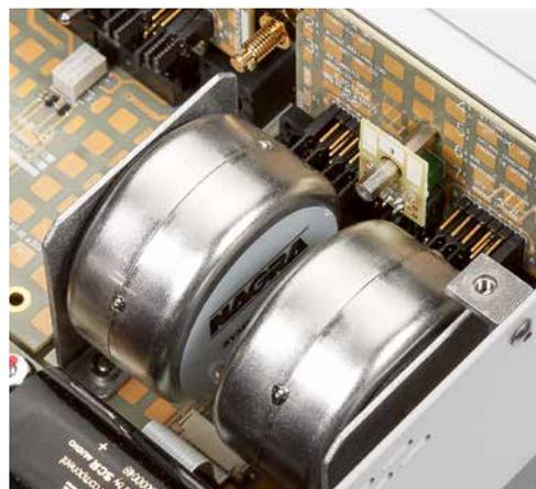
The small plug-in board for MC resistance adjustments sits between the two transformers. In this case we had chosen 270 ohms.
