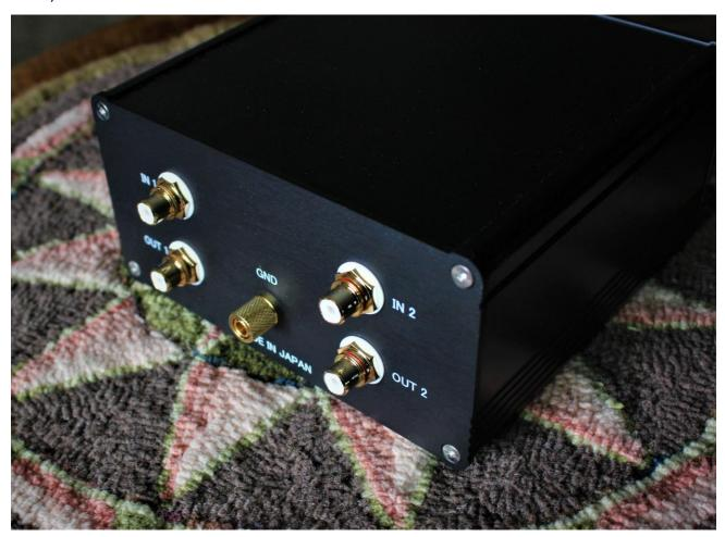
The Koetsu SUT is custom made for Koetsu cartridges. It adds 26 dB of gain, and it's designed to be the perfect load for Koetsu cartridges. I used the SUT with other cartridges I had on hand such as the Hana Umami Red, Sumiko Celebration 40, Allnic Audio Amber MC and a few more—and it most cases the sound was different but not necessarily better. With the Koetsu Urushi Black and the SUT, the improvements were more than obvious.
