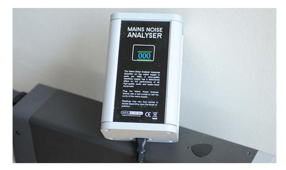
ever growing problem with our power lines around our homes. There we have two types of mains noise. Common mode is usually referred to as RFI and differential mode is created when components draw power."
