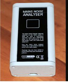
The Mains Noise Analyser measures stortion on the mains supply in parts per 1000. A poor-quality electricity supply has a detrimental effect on the performance of all high-quality audio and audio-visual equipment.
