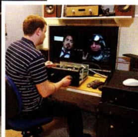
LEFT and BELOW: Checking one of the first SPA22 AV amplifiers, comparing it against Primare's references. Construction is modular, allowing for planned upgrade 'cards' to be slotted in
