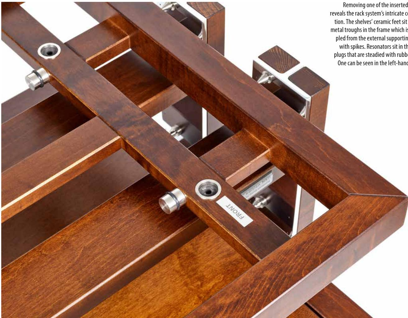
Removing one of the inserted shelves reveals the rack system's intricate construction. The shelves' ceramic feet sit in small metal troughs in the frame which is decoupled from the external supporting frame with spikes. Resonators sit in the metal plugs that are steadied with rubber rings. One can be seen in the left-hand image.
