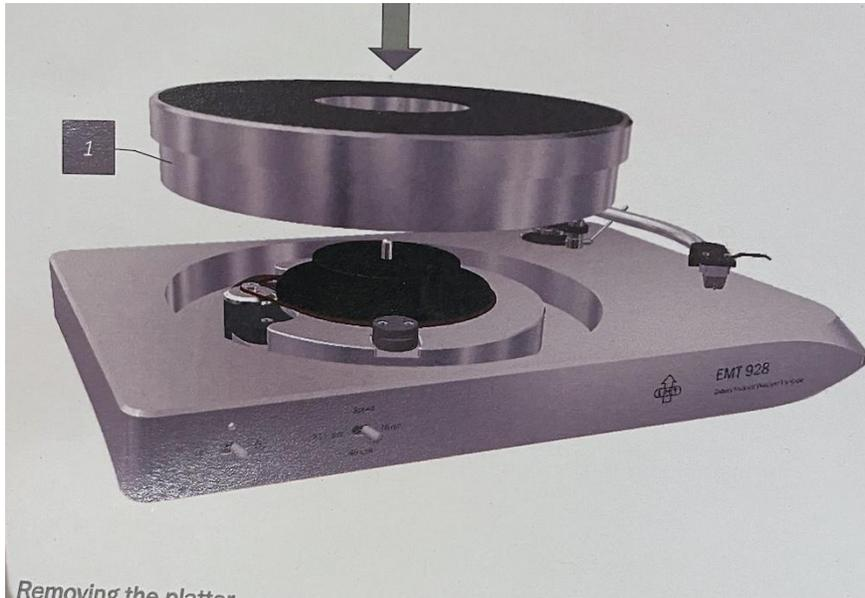
weighs fifty pounds (the Thales 'table pictured above weighs roughly half as much)! Much of the stepped platter is hidden within a circular recess in which is a stepped sub-platter upon which it rides (I'm using the instructions' illustration rather than removing the top to take a picture).
