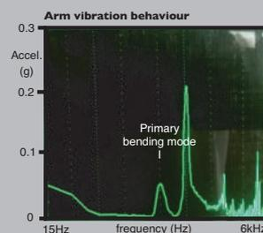
The carbon fibre arm was unusually well damped, with no sign of a first order bending mode around 200Hz – unusual. It is also stiff, the first visible bending mode being at a high 500Hz.
