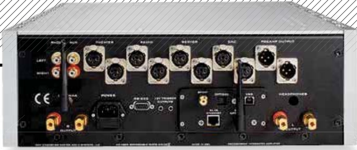
ABOVE: Fully loaded, the amp offers four balanced line ins on XLRs, one MC phono and a line in on RCAs. Antenna [left] is for the BT remote, the other for wireless Wi-Fi alongside Ethernet, USB-B, coaxial and optical digital ins. Outputs include 4mm speaker binding posts, one balanced pre out (on XLRs) and a 6.35mm headphone out
