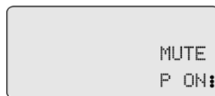
Display in operating condition PROTECT ON
