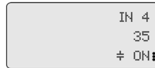
Display in operating condition ON, DC-protection active
