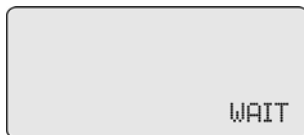
Display after switch in of the mains
