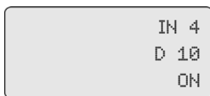
Display with active Volume-Dim function
