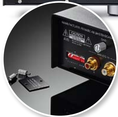
ABOVE: Single phono inputs [far left] are switched between MM/MC by a toggle, alongside other toggles for gain and subsonic filtering. Input loading DIP switches are hidden behind small panels [inset]. RIAA eq'd outputs are offered on RCAs and balanced XLRs
