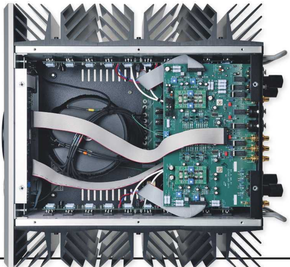
RIGHT: No fewer than ten pairs of power MOSFETs are deployed on massive heatsinks per channel and with sufficient standing current to support a claimed 16W in Class A mode
