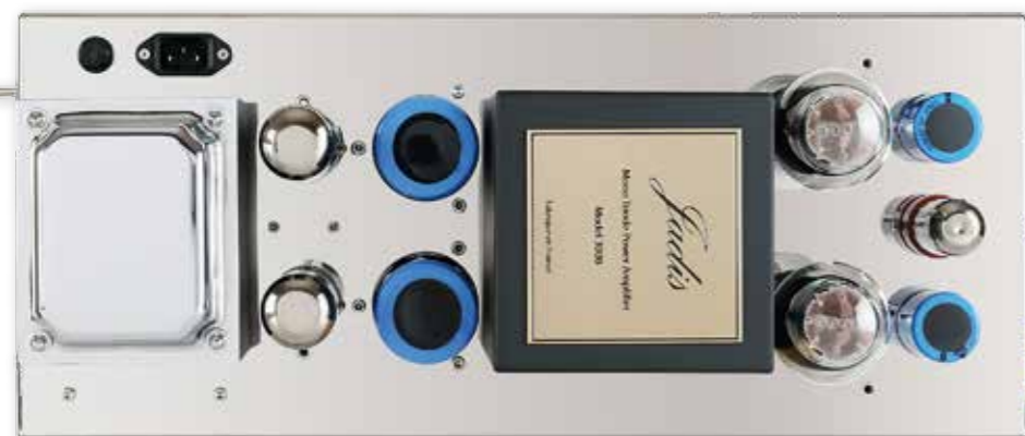
LEFT: The Jadis SE300B seen from above showing, from left to right, the AC mains transformer, a pair of 5U4GB rectifier tubes and PSU caps, the custom resin-potted output transformer, paralleled 300B triodes and single 6SN7 driver tube
