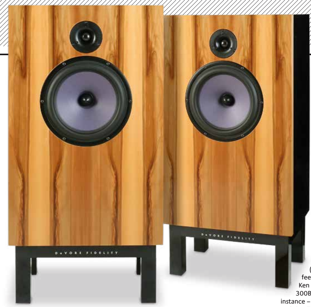
LEFT: The O/96's fibreboard cabinets are fronted by a 1in-thick US-made Baltic birch baffle. The 250mm bass/mid unit features a Kurt Müller blue paper cone, joined here by a 28mm silk dome
